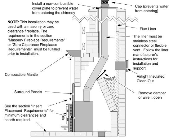
Insert with Direct Connection (Masonry Fireplace)
