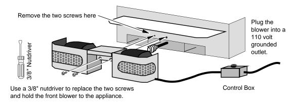
2. Plug the power cord running from the control box into a grounded 110 volt electrical outlet.
