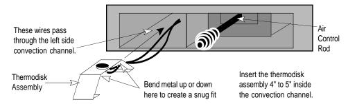
Install the wire clip following the directions below.
