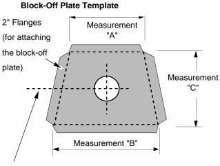
The center of the flue is 9 1/4" back from the fireplace opening (6 1/4" in diameter).
