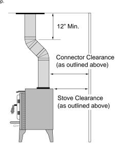
Standard Ceiling with a Factory Built Chimney
